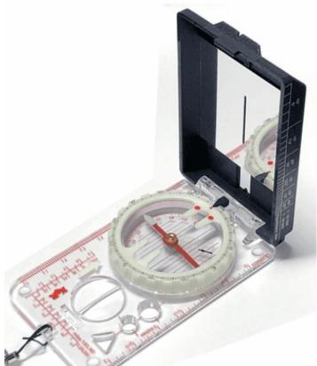
**Figure 1.** K&R Alpin Sighting compass with inclinometer.
